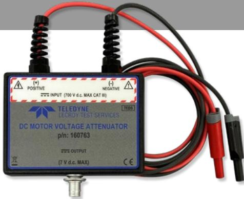
The Teledyne LeCroy Test Services Motor Voltage Attenuator (MVA) products are used to measure motor voltages on 3-phase AC inductive and DC motors. The MVA's use precision attenuators that convert high level AC/DC voltage to low level signals that can be input to the QL3-FS system.
