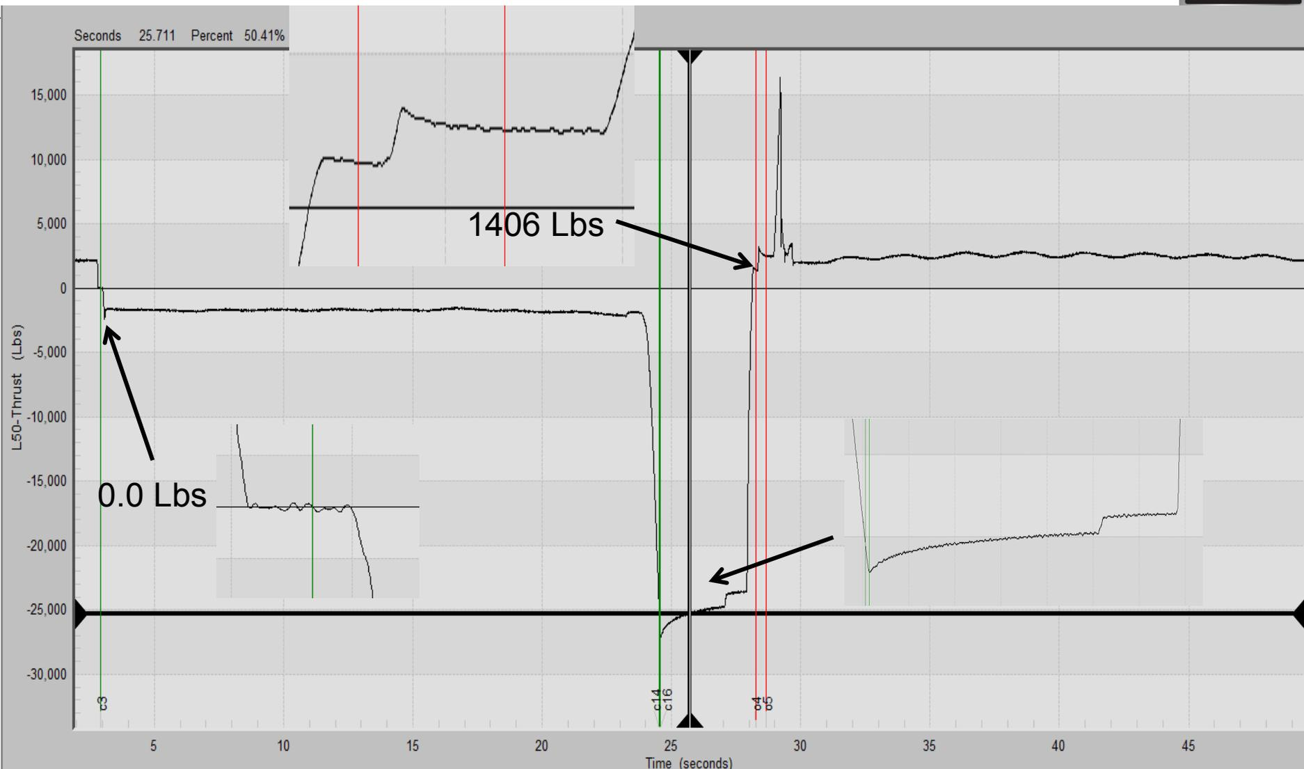
There is 1406 lbs difference between c3 and 04 and thrust releases after c16.
