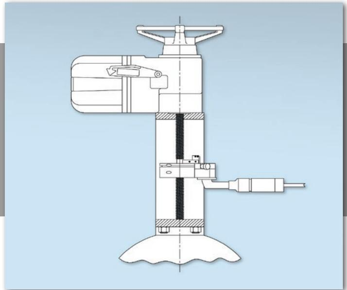
The Thread Removal Tool is used for the in-situ removal of valve stem threads. This permits the installation of Teledyne Test Service's Quick Stem Sensor (QSS) on a smooth stem area for direct, accurate measurement of stem torque and thrust. A procedure for use of the thread removal tool is supplied.
